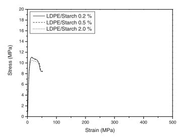
Figure 2. LDPE/starch blends mechanical properties after 120 days of exposition time.
